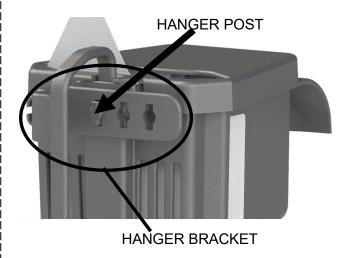
Place the hanger bracket at 90° and align one of the adjustment holes onto the mounting post as shown in the illustration **ABOVE**.
